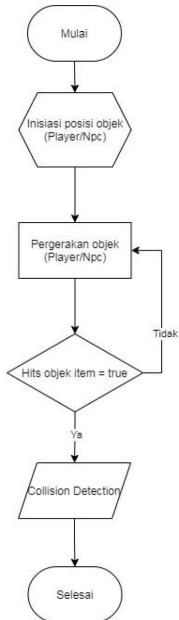
**Gambar 1. 3 Flowchart Collision Detection**
