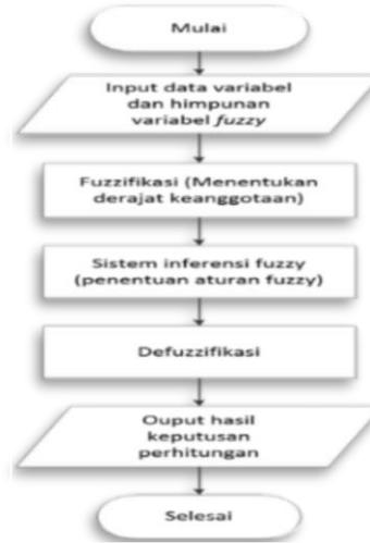
**Gambar 1. 2** Flowchart Algoritma Fuzzy Logic Sugeno
